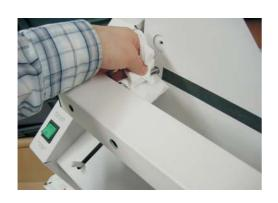
2) CLEAN GUIDE RODS from oil or lubricants. Remove clamp from guides if necessary. Clamp works optimally with VERY little amount of oil. Use solvent for cleaning if necessary.
