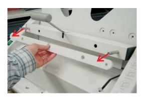
1) REMOVE SUPPORT rod. Open to screws with hexagonal key.
