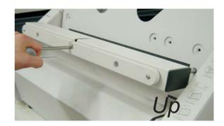
10) Check that clamp moves smoothly from down to up position. If clamp is too tight, it does not move smoothly up. Then loosen adjustment screws.
