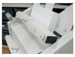
6) Clamp strength test: take a 30 - 50 mm thick block of 80g normal copy paper. Place the block to the clamp. Lock and close the clamp.
