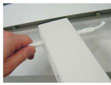
3) CLEAN BOTH LOCKING UNITS (inside the clamp) from oil and lubricants. Clamp works the best with none or VERY little amount of oil. Use solvent if necessary.
