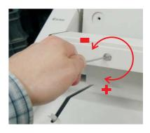
Tighten clamp: turn clockwise Loose clamp: turn counter clockwise.
