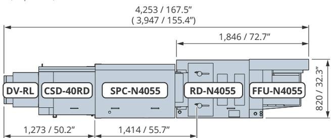
\*Inside ( ) is the dimension when using the normal tray.
