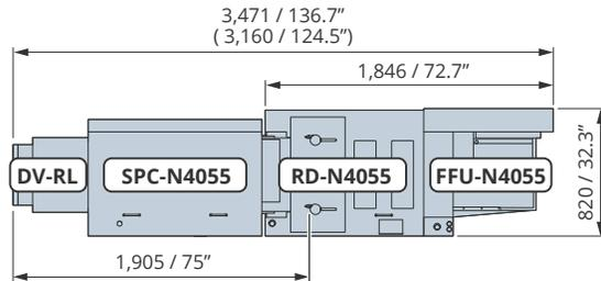
\*Inside ( ) is the dimension when using the normal tray.
