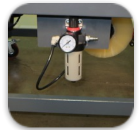
Air Required for Pneumatic Minor Flap Closer
