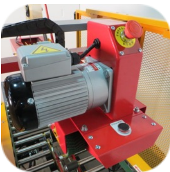
2 Top Drive Belts with ¼ HP Motors and Emergency Stop Switch
