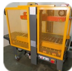
Fully Enclosed Safety Gates Will Shut Machine Off if Opened
