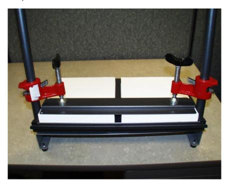
5. Allow the compound to dry for 10 to 20 minutes. Loosen the clamps and slide them out of the way. Remove the clamp bar and pads. Wipe compound from the lower door slot after each use.
