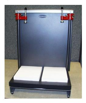
2. Place the clamp on top of the piles as shown. Slide the pipe clamps down the vertical bars. Firmly tighten the screws onto the clamping bar.
