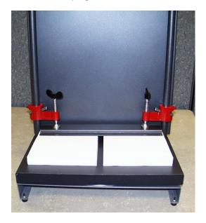
3. Rotate the table 1800 in either direction until the table locks into place.
