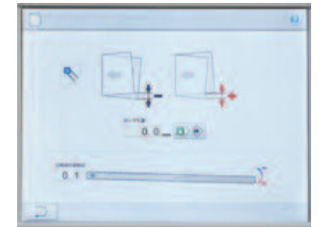
Fine-adjustment for skewed folds sets automatically by entering the skewed fold measurement or shift amount of the sheet register guide.
