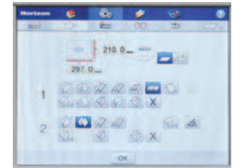
Setup is completed by selecting the desired fold pattern and inputting the sheet size.
